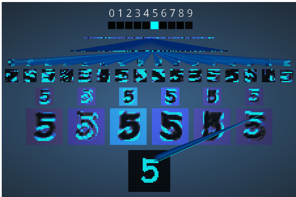
Figure 7: A visual representation of a convolutional neural network for digit classification 4 . The bottom layer are convolution layers for convolutions and subsampling, while the top layers are fully-connected layers.
